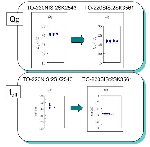
(Same Maximum Ratings in  $V_{DSS}$ ,  $I_D$ ,  $R_{DS(ON)}$ )
